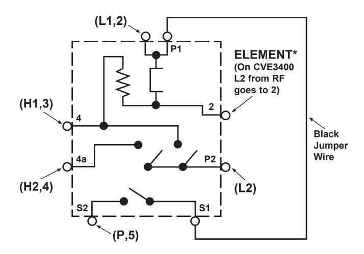
\*On units with a compound connection, the two red wires must be separated. Locate the right front switch connection (L2). The red wire routed from the right rear element/switch will remain, but the red wire routed from the left rear element/ switch must be disconnected, reterminated and connected to position 2 on the new dual switch.
